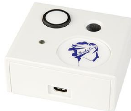
Activation box to turn on the capsule
